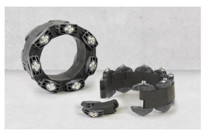
Besides the classical advantages of a modular sealing system, Hauff-Technik is offering additional benefits. When using the modular seal on lager pipelines a multitude of segments has to be used. In such cases installation takes some time as it is necessary to tighten each and every bolt several times. Easily one segment can be overlooked and/or not tightened enough.
