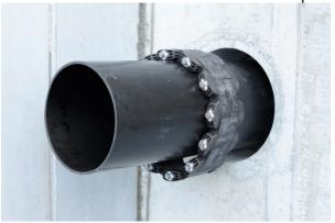
The modular sealing system from Hauff-Gliederkette allows to seal with only 12 different segments sizes pipes from diameter 48,3 to 2.000 mm and an annular space between 19.5 and 98 mm.
