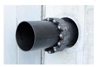
The modular sealing system from Hauff-Gliederkette allows to seal with only 12 different segments sizes pipes from diameter 48,3 to 2.000 mm and an annular space between 19.5 and 98 mm.
