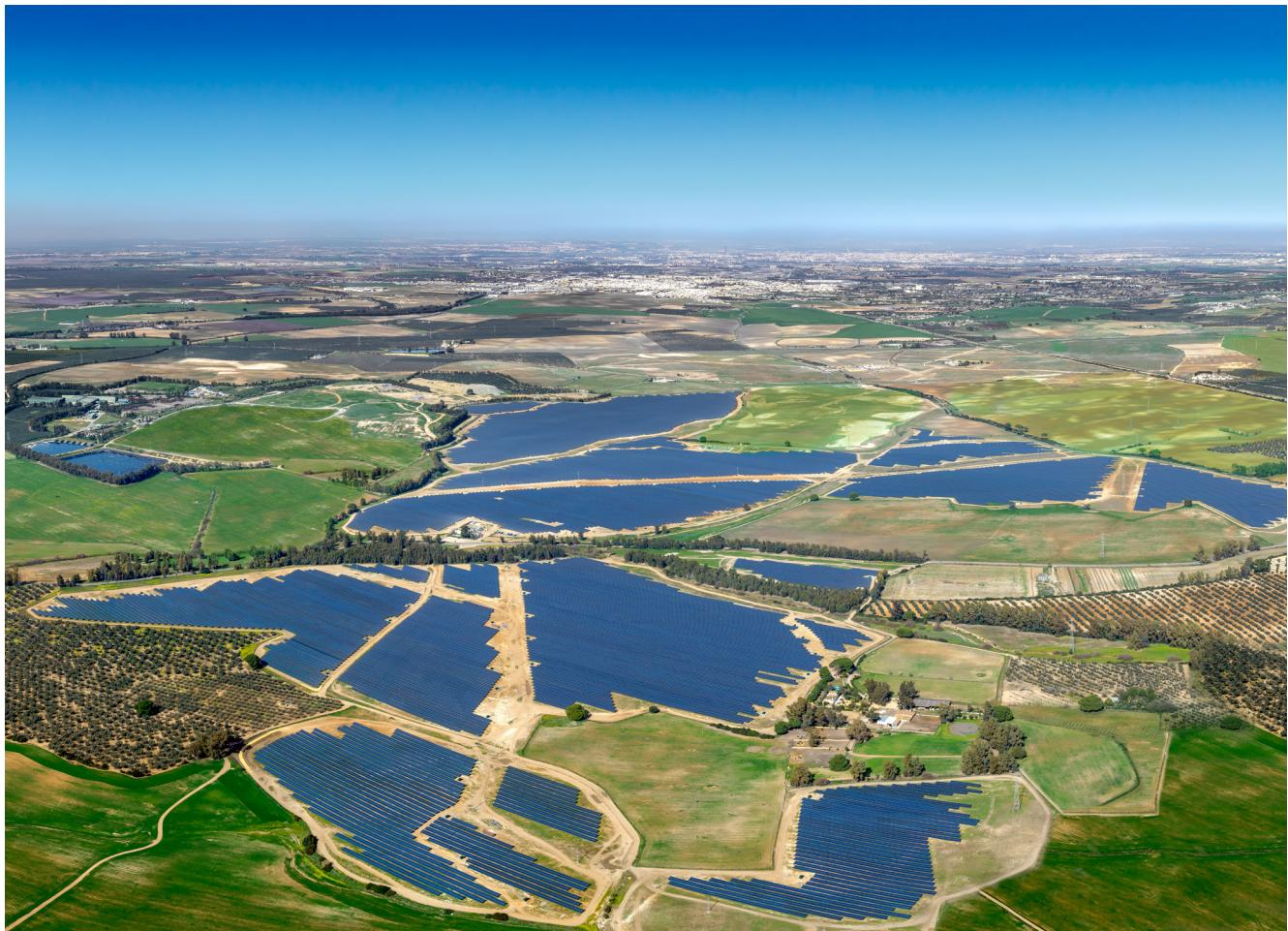
POSTAVLJENO JE VIŠE OD 500 000 SOLARNIH MODULA NA POVRŠINI OD 265 HEKTARA
